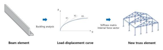
2.1 A Data-driven truss element
